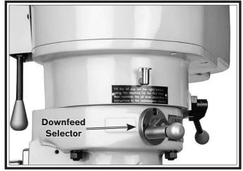
Figure 36. Downfeed selector in the manual (disengaged) position.
